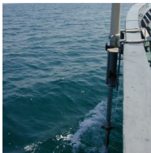
Fig. 2. Mounting of the probe to the support (left) and probe attached to the boat (right)
