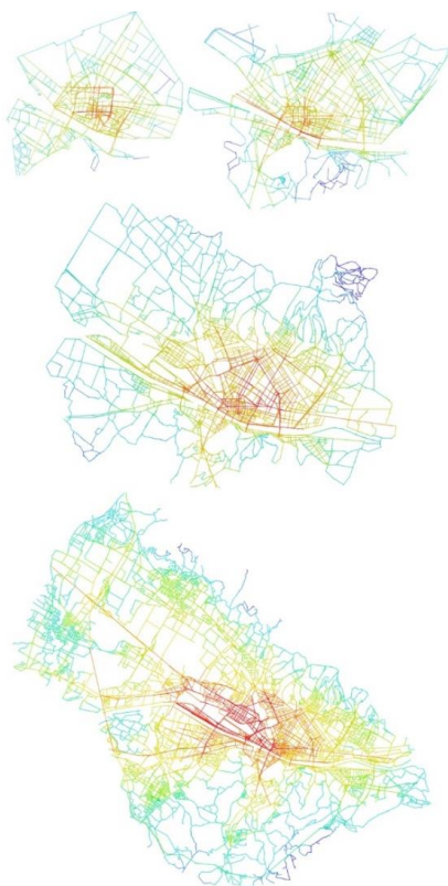
Figure 1 - The distribution of integration value in the grid of Florence at 1825 (top, left), 1910 (top, right), 1955 (middle) and 2015 (bottom)
